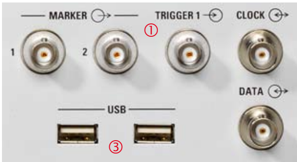
Trigger input and marker outputs on the front panel of the R&S® AMU200A
